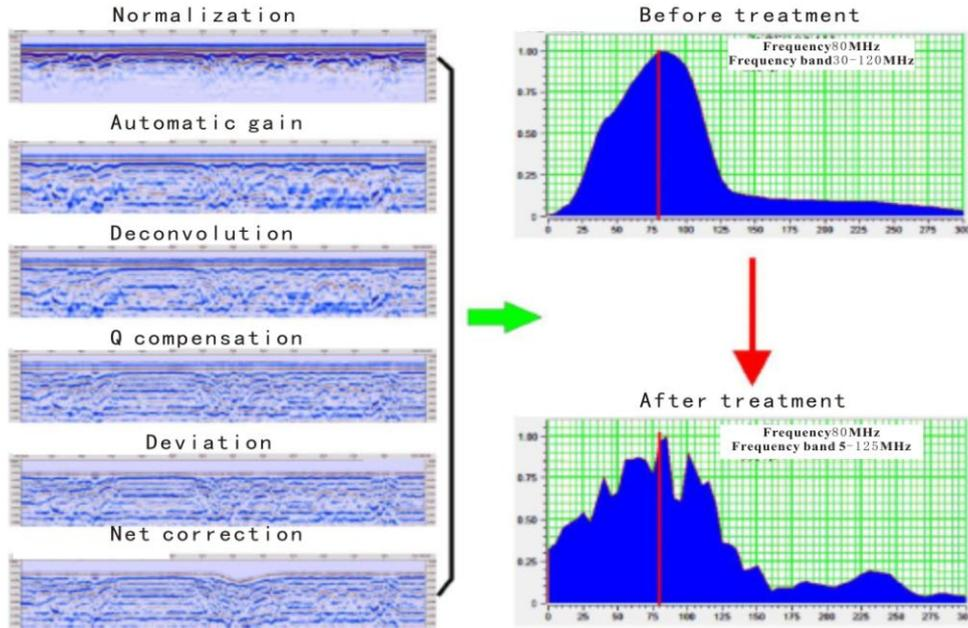
**Fig. 2** GPR data processing flow
